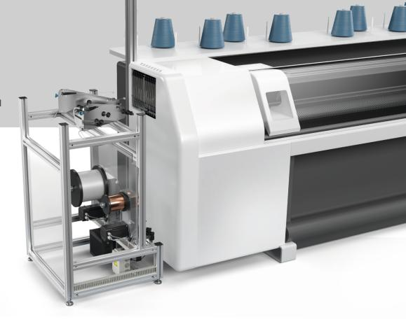
The MTD is a positive drive for flat knitting machines where the material is unspooled in radial (tangential) instead of axial (over-head) direction. This enables twist-free unspooling of the material to be processed.
