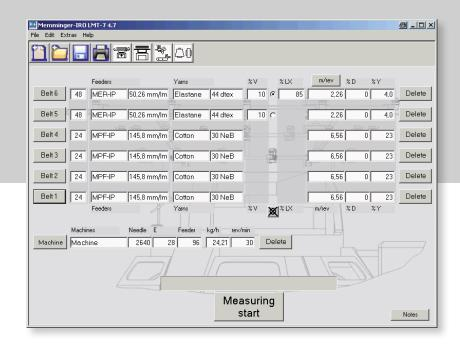
The LMT 7 is an electronic, software-based yarn infeed meter. It collects and processes production data from circular knitting machines operating with continuous, positive feed of basic yarn with or without elastane.
