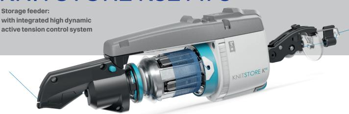
KNITSORE K52 ATC combines all the advantages of the basic storage feeder KNITSTORE K52 such as functional design, easy maintenance and operation with the high dynamic active tension control system (ATC).
