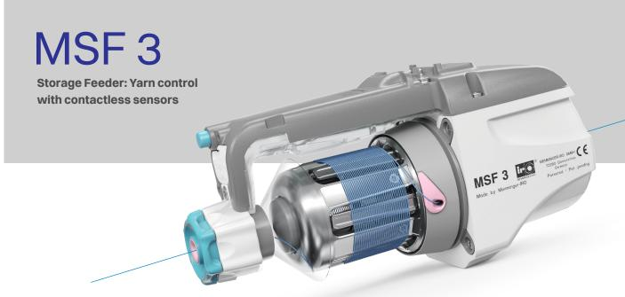
The MSF 3 Storage Feeder has a stationary winding body and a yarn winding transport system. It has been designed for the feeding of yarn at constant and variable feed rates to knitting and hosiery machines.
